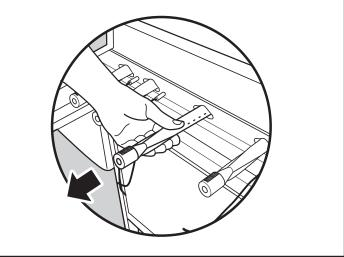
15. To reinstall the manifold assembly, reverse steps 7 through 14. **CAUTION: The burner openings (1) must be positioned**
