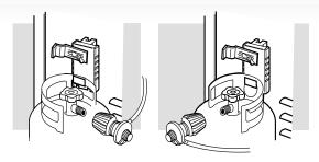
Loosen the cylinder lock wing nut. Swing the cylinder lock down. Tighten the wing nut.
