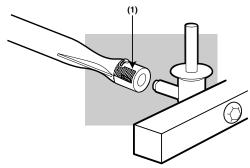
We recommend that you inspect the Spider/Insect screens at least once a year. (See Section "Annual Maintenance".) Also inspect and clean the the Spider/Insect screens if any of the following symptoms should ever occur:
