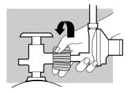
Note: This connection tightens clockwise and will not allow gas to flow unless the connection is tight. The connection requires tightening by hand only.
