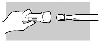
Clean the inside of the burners with a wire (a straightenedout coat hanger will work). Check and clean the air shutter opening at the ends of the burners. Check and clean the valve orifices at the base of the valves. Use a Steel bristle brush to clean outside of burners. This is to make sure all the burner ports are fully open.
