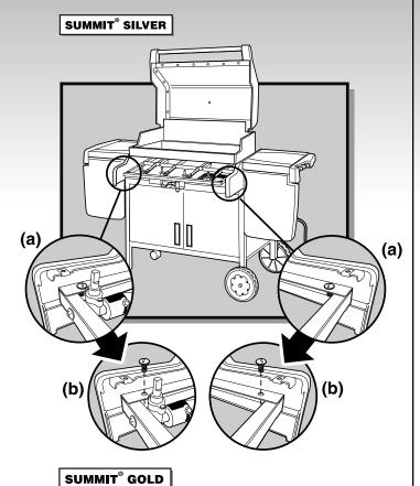
10. Pull manifold assembly out from the manifold frame.
