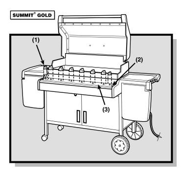
Put your fingers under the front edge of the control panel and lift off.
