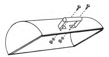
12. Set the HOOD, in the CLOSED POSITION, on top of the bottom Half of the grill body. Line up the Hinge holes and insert the Hinge Pins. This may require lifting up on the back of the Hood. Then, carefully open the hood, making sure to not let the Hinge Pins fall out, and insert the Hair Cotter Pins into the Hinge Pins. See below.
