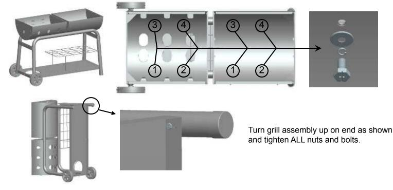
Attach the CATCH PAN to the underside of the GRILL BODIES using two (2) <sup>1</sup>/<sub>2</sub>" BOLTS as shown. Insert the BOLTS down through the GRILL BODY and then screw into the CATCH PAN. Make sure that the side of the catch pan marked "Wheel Side" is on the side of the grill with the wheels. From the rear of the grill, slide the GREASE TRAY into the guides/rails under the CATCH PAN.
