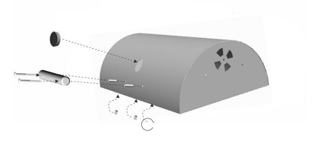
Place top assembly on top of bottom assembly. Align hinge hole on back of unit. With aid of a helper attach hinges to top Assembly using (4) 1/4-20x1/2" hex screws.
